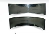
Localized excessive wear of the bearing surface along the bearing edge. Possibility of fatigue cracks in the affected area.
